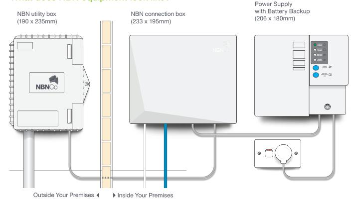
The NBN connection box shown is designed for use inside the home and business. If your installation requires an external NBN connection box your device will differ to the one shown above.
